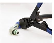
5. Close the clips using the crimping tool (part # 54-11380). The pliers will open themselves when clip is fully crimped. Crimp the clip closest to the fitting first.
