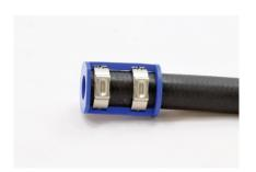
3. Insert hose into clip holder with the clips.
