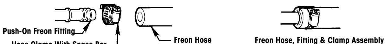
Figure 3 – PUSH ON FITTING (R-12 SYSTEMS ONLY)
